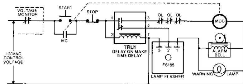
**Delayed Restart:** When line conditions return to normal, the relay contacts in the PLM voltage monitor close. The TRU'S restart time delay begins. The alarm sounds, warning operators of pending restart. At the end of the delay, the contacts in the TRU transfer, starting the motor and extinguishing the alarm.
