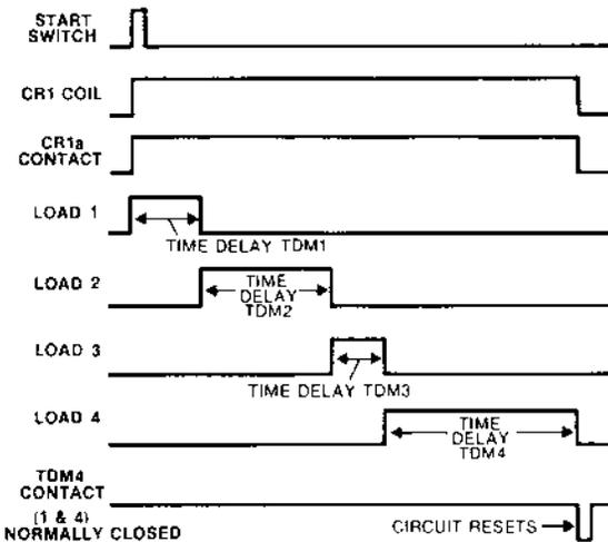
**Staging (ON and OFF):** On closure of SW1, Load 1 is energized and a time sequencing ON condition is initiated. At the end of the T1 ON delay, Load 2 is energized which in turn initiates the ON delay of timer T2. When the second ON delay is completed, Load 3 is energized. Additional TDMB Time Delay Relays can be connected to operate additional loads. With the opening of SW1, each load in the system is sequenced OFF starting with Load 1 and continuing with Load 2, then Load 3.
