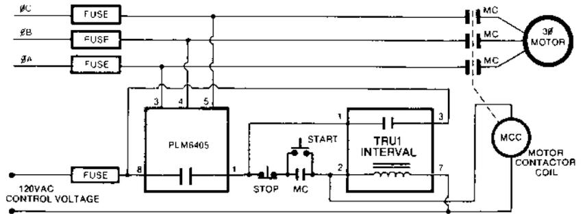
**Compressor Anti-Short Cycle Lockout Delay:** The anti-short cycle time delay prevents locked rotor starts by locking off the compressor contactor until internal pressures have equalized. Should the PLM voltage monitor sense a line fault, its open contacts will start a lockout delay. The compressor cannot restart until the line fault is corrected and a five minute delay is completed.
