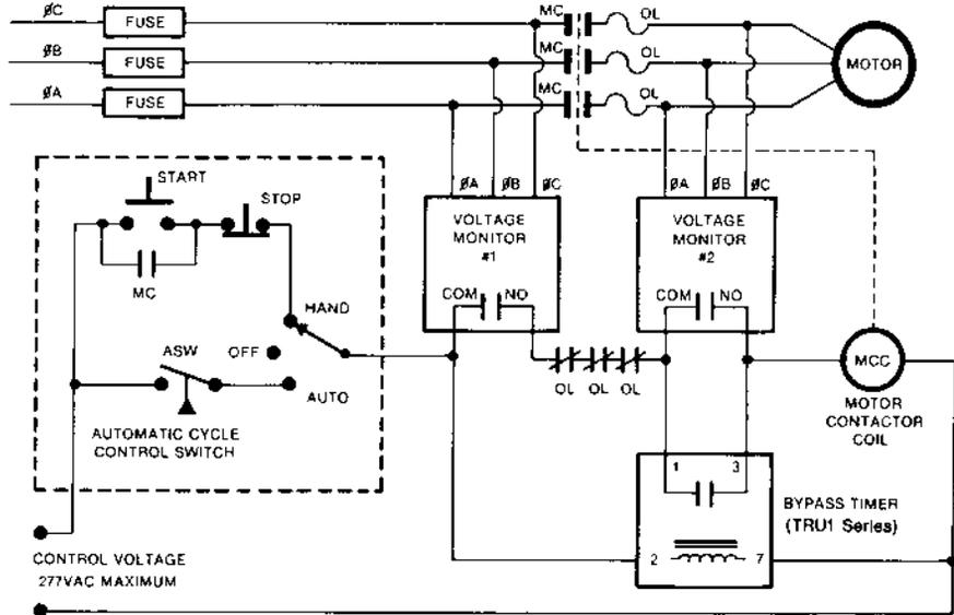
voltage monitors and bypass timers are installed in each motor control panel and connected like voltage monitor #2 in the diagram. The RLM, TVM and TVW series are good choices for the load side monitor because of their superior protection from the high voltages caused when the contactor disconnects the rotating motor.
