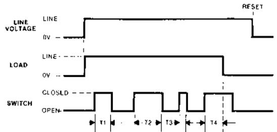
$$T1 + T2 + T3 + T4 = \text{Total Preset Time Delay (Determined by } R_T)$$
