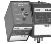
Provides equal run time for two loads. Automatically changes lead load upon the opening of the control switch input. Industry standard wiring.
